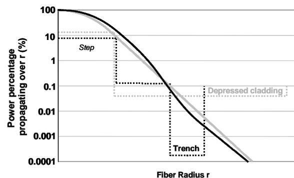
*Figure 1: Profiles (dotted lines) and percentage of mode power propagating over radius  $r$  (full lines) for trench-assisted (black) and depressed-cladding (gray) step-index profiles*
