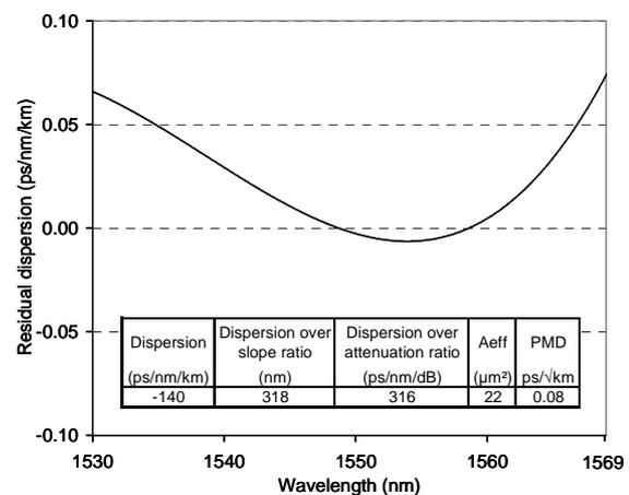
Figure 2: Residual dispersion of LAF+DCF link (inset: characteristics of the DCF at 1550nm)
